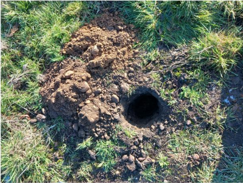
Photo No.9: WS05 located in the NE of site and showing the inspection pit (drilling refused here on sandstone cobble)
