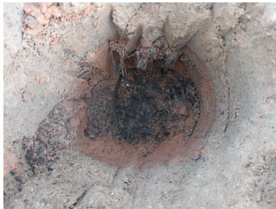
Photo No.6: IP03 pit sides and base showing ménage sand material atop membrane atop ashy subbase
