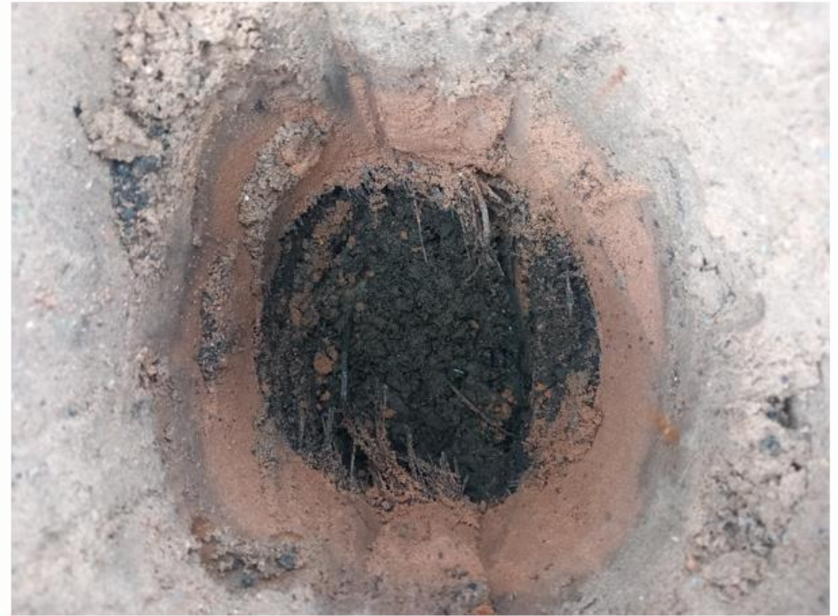
Photo No.8: IP04 pit sides and base showing ménage sand material atop membrane atop ashy subbase
