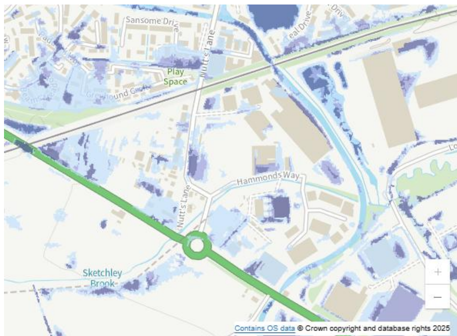
Figure 3.2 Surface Water Flooding Extent Map (Courtesy of gov.uk)
