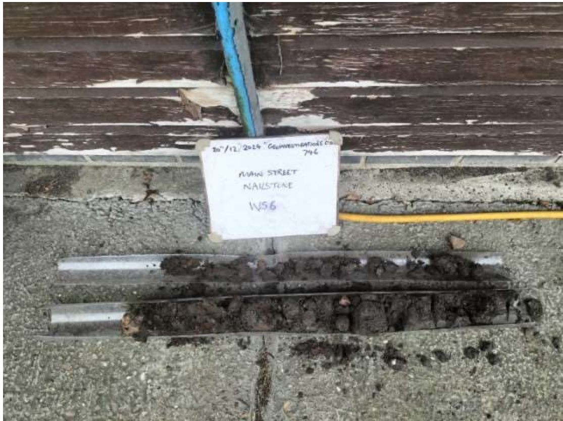
Borehole WS6 soil core to 1.0m begl.
