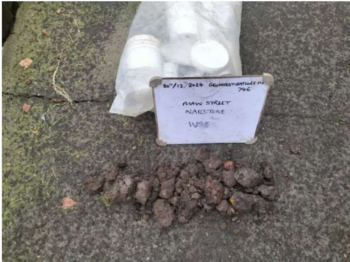
Borehole WS5 soil core to refusal at 0.50m begl.
