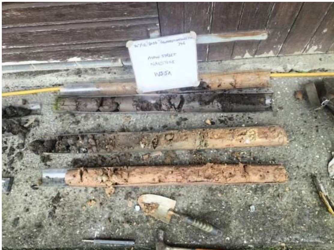
Borehole WS5A soil cores near centre of the pond.
