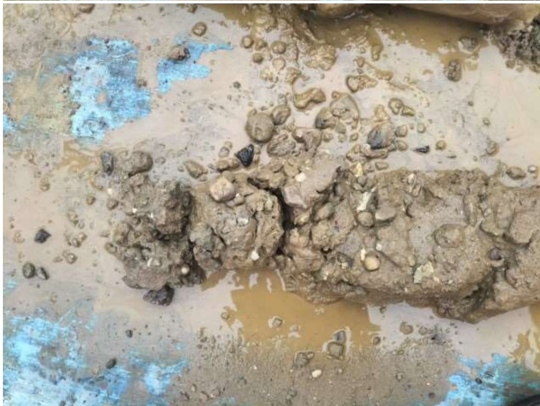
Borehole WS2 soil cores, including close-up of typical very clayey, very sandy gravel encountered.
