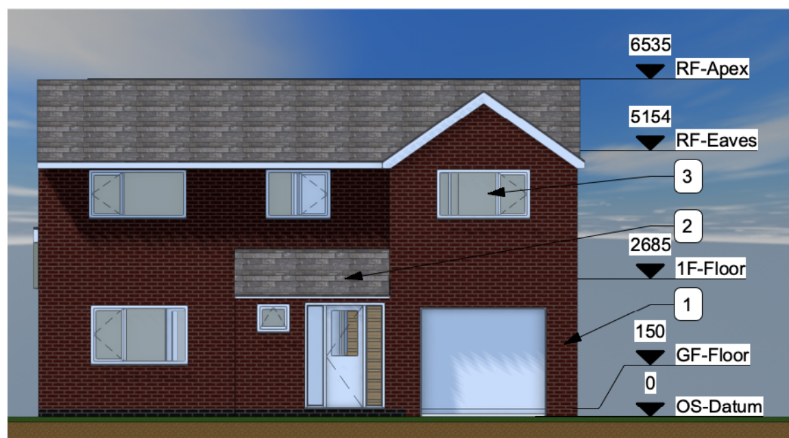
1 South Elevation - Proposed Scale: 1:100
