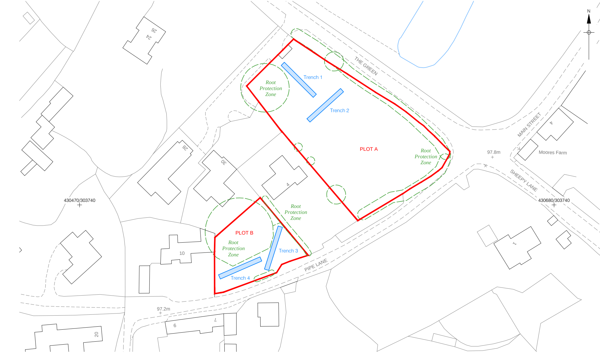
Figure 2 Detailed Site Plan showing Proposed Trench Locations and Root Protection Zones 1:1,000 at A4
