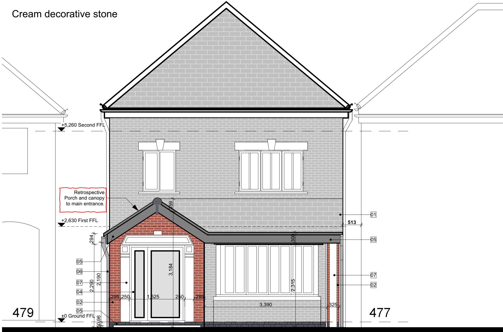
As-Built Front Elevation
