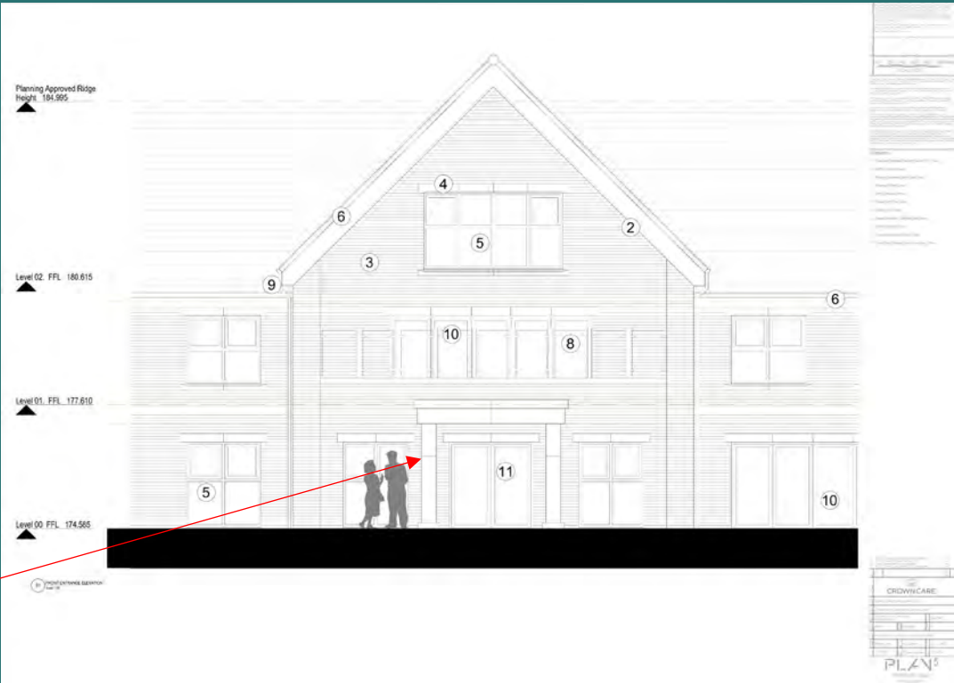
Portico at front entrance
