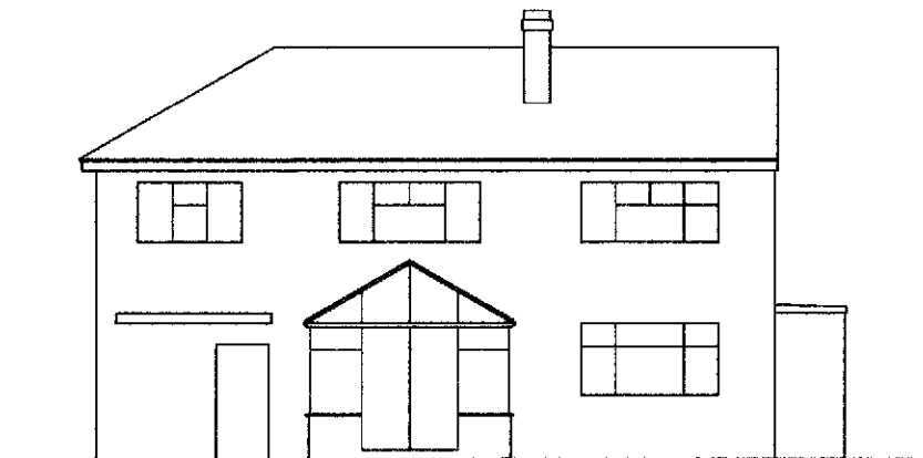
existing rear elevation
