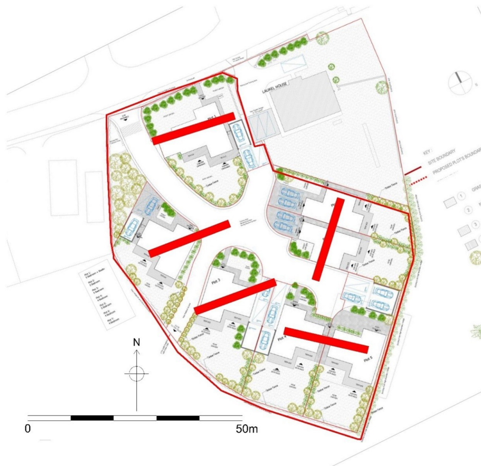
Figure 5: Location of trenches (red) with site outline (red) (supplied by client).
