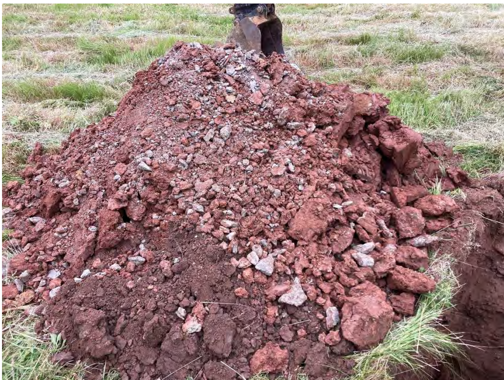
Trial Pitting note siltstone fragments
