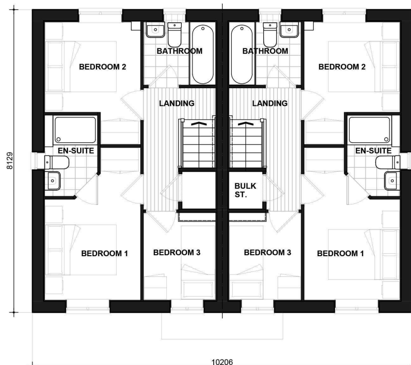
CL389 FIRST FLOOR PLAN
