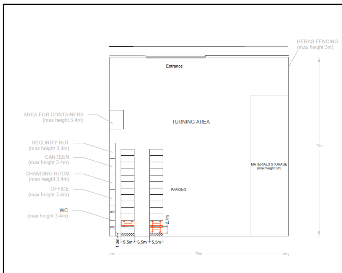
Figure 4: Large Temporary Construction Compound
