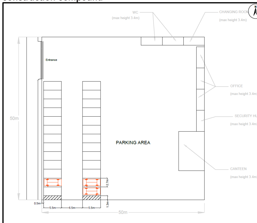
Figure 12b: Parking of Site Operatives and Visitors Vehicles at 50m x 50m construction compound
