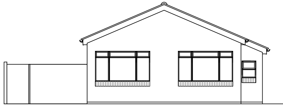
Existing Front Elevation @ 1:100
