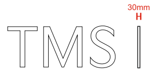
Sign 'D' Scale 1:50 Size: 545mm Cap height illuminated white acrylic Surface mounted dealer name letters - 30mm depth Height from ground level = 3500mm Span of text = 1418mm
