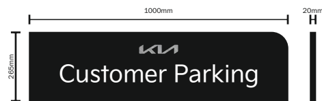
Sign 'G' Scale 1:20 Size: 1000mm x 265mm x 20mm Description: 20mm composite with anodised face to logo non illuminated Cap height of 'P' in 'Parking' = 90mm Logo Height = 35mm Height from ground level = 1250mm
