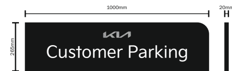
Sign 'H' Scale 1:20 Size: 1000mm x 265mm x 20mm Description: 20mm composite with anodised face to logo non illuminated Cap height of 'P' in 'Parking' = 90mm Logo Height = 35mm Height from ground level = 1250mm
