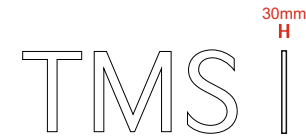
Sign 'C' Scale 1:50 Size: 545mm Cap height illuminated white acrylic Surface mounted dealer name letters - 30mm depth Height from ground level = 3500mm Span of text = 1418mm
