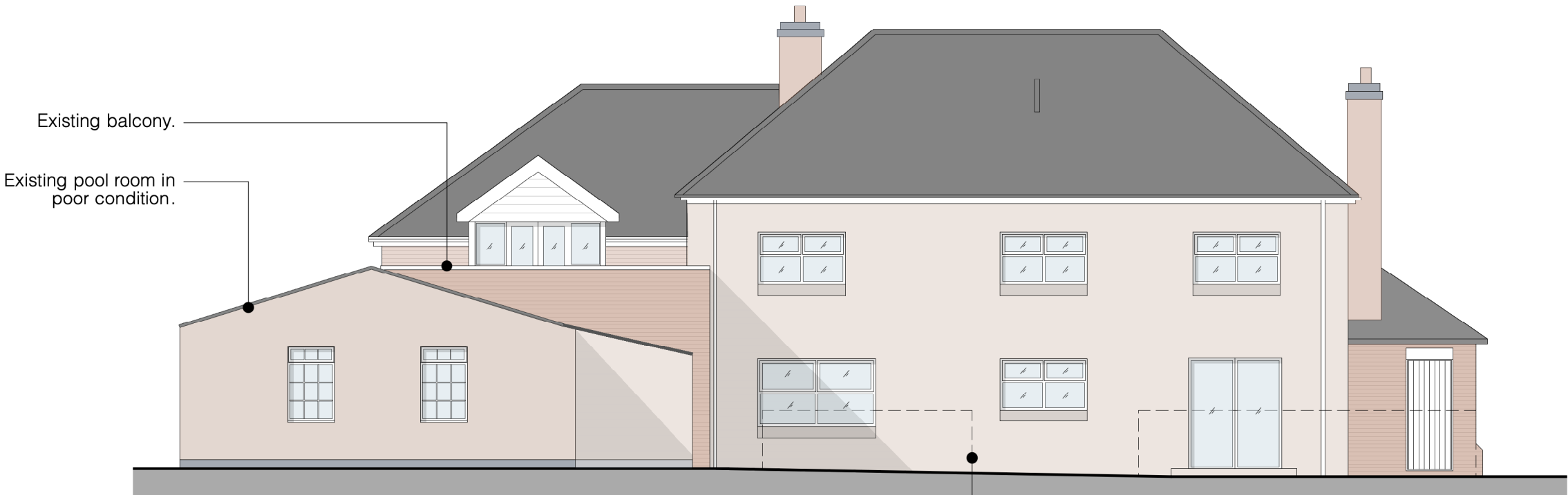
2 existing rear elevation (south)
