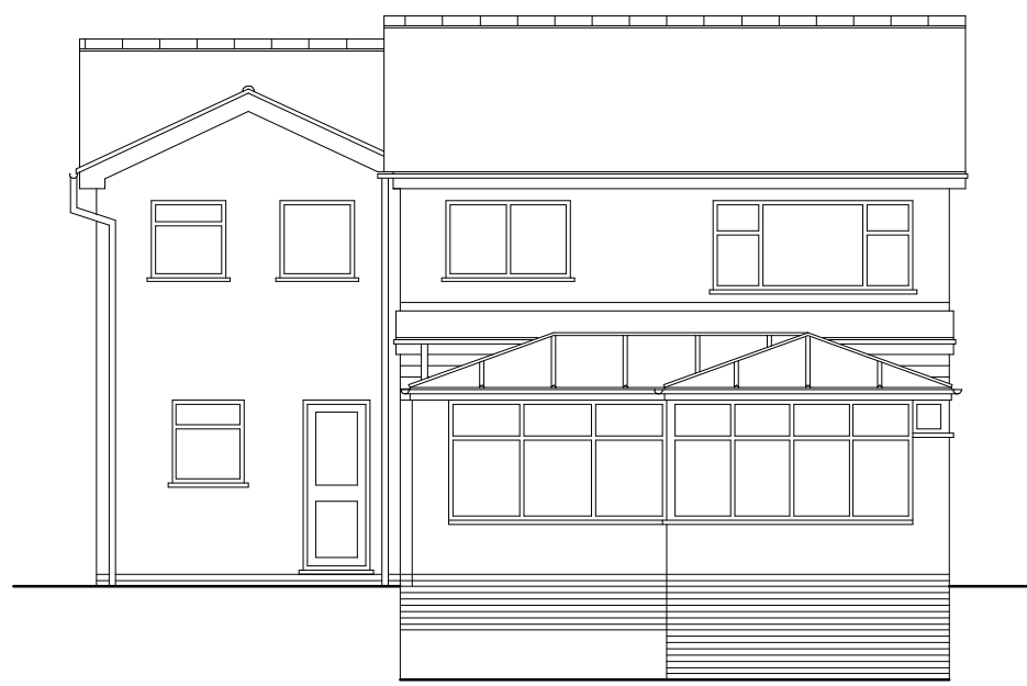
Existing Rear Elevation
