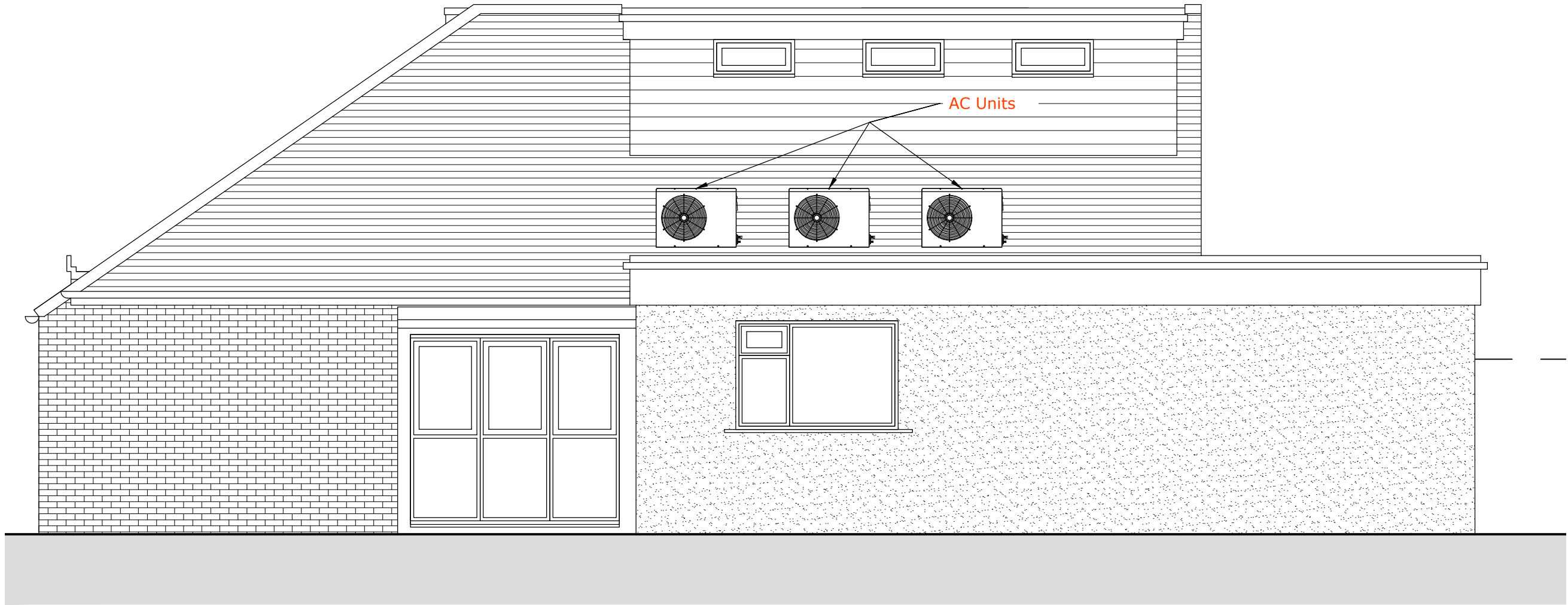
North Elevation as EXISTING 1:50
