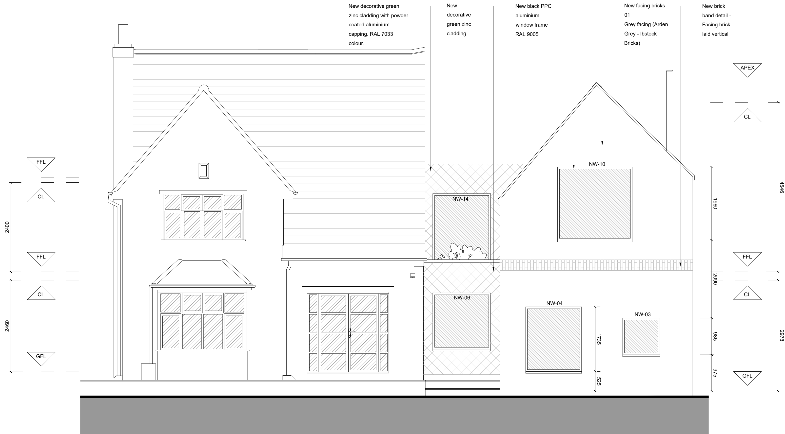
Elevation B (Rear) Scale 1:50
