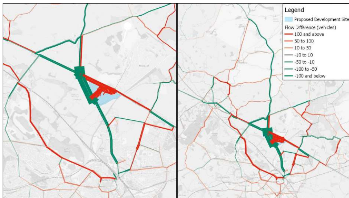
Figure 3.1: Forecast Flow Change for 2031 'With Development' minus 'Without Development'
