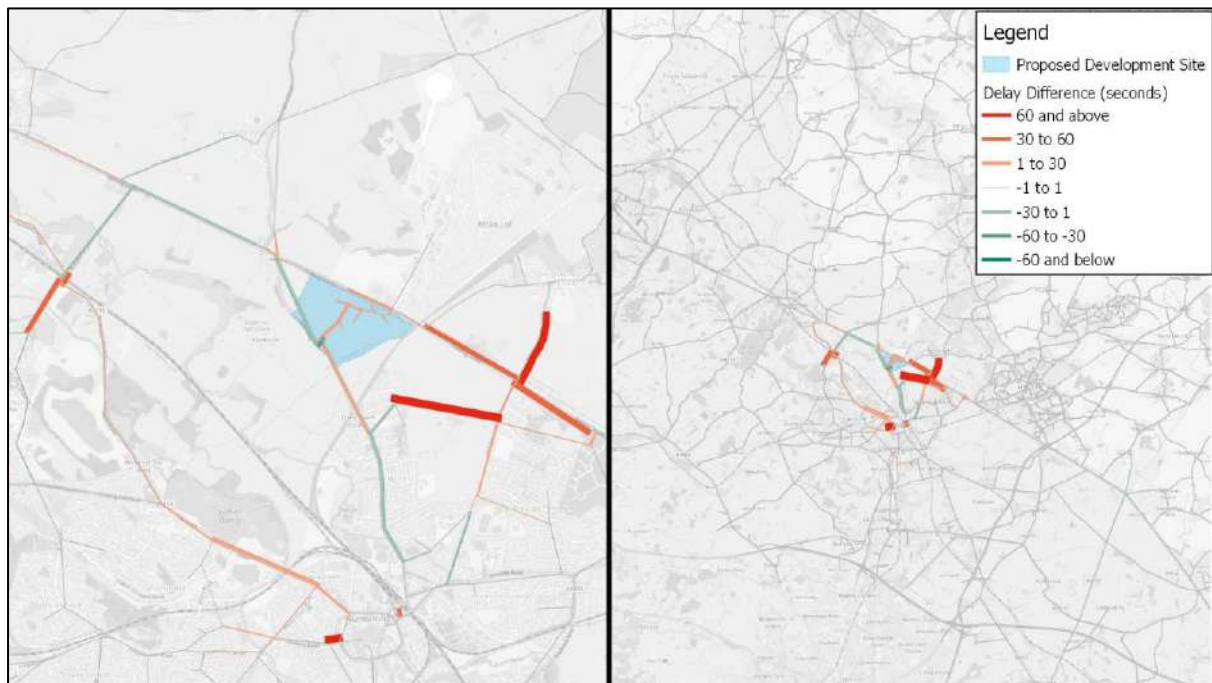
Figure 3.3: Forecast Delay Change for 2031 'With Development' minus 'Without Development'
