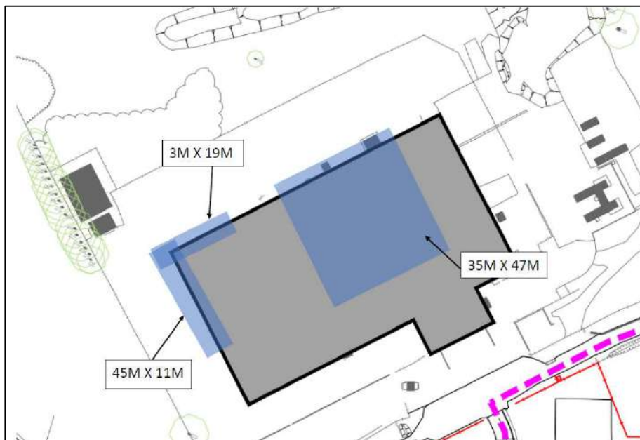
Figure 4-1 Location of ACMs under Building 1 footprint
