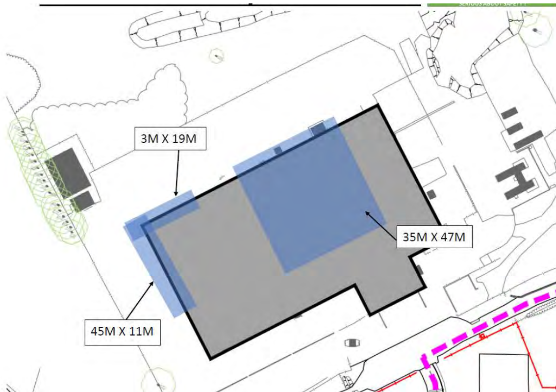
Figure 1 – Approximate Locations of ACMs under building footprint
