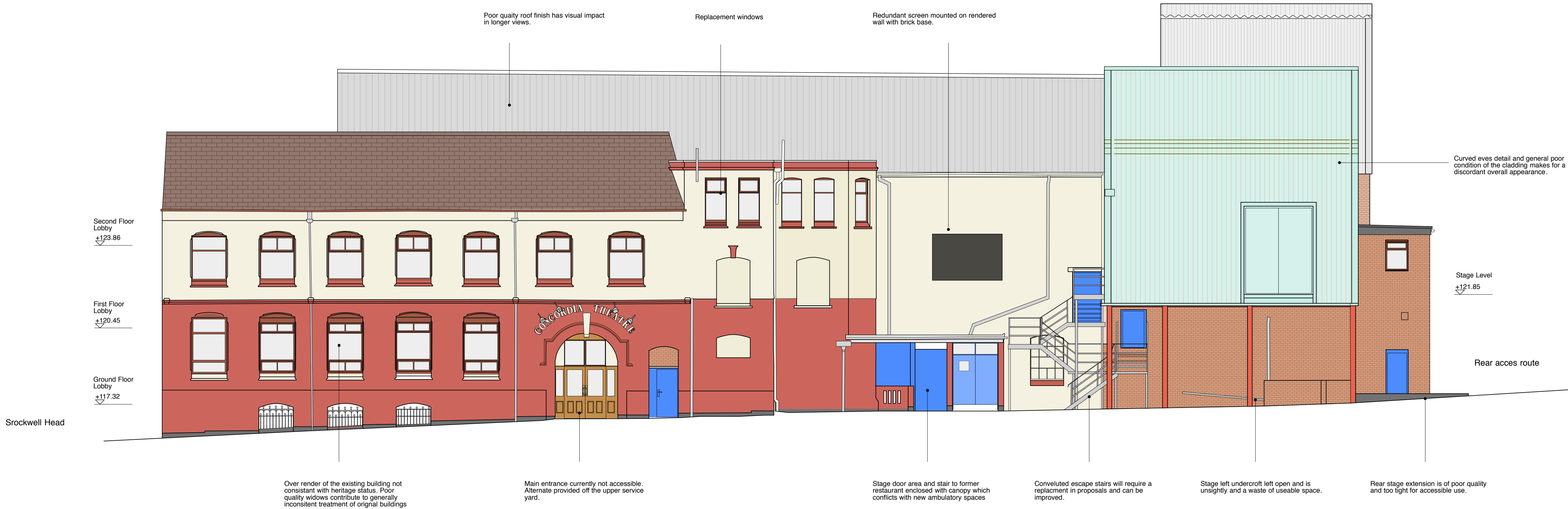
SOUTH-EAST ELEVATION : AS EXISTING
