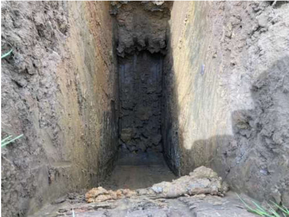
TP48 – Trial Pit
