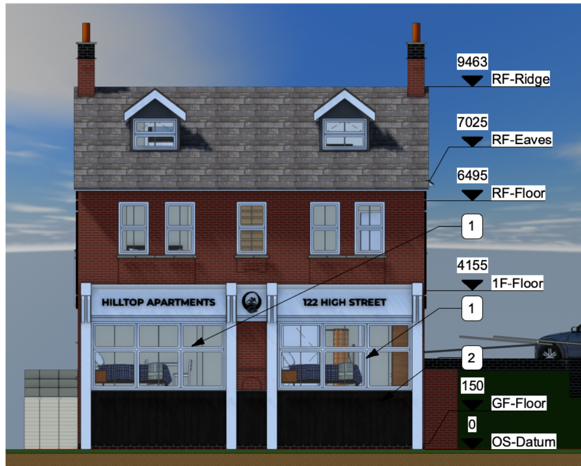
1 South Elevation - Proposed Scale: 1:100
