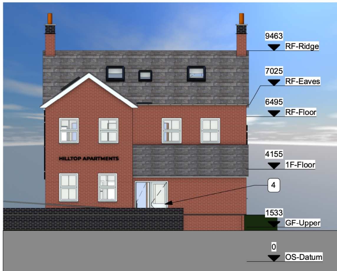
3 North Elevation - Proposed Scale: 1:100
