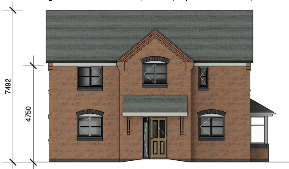
Figure 11: Front Elevations, Units 4 and 5 (Hayward Architects)
