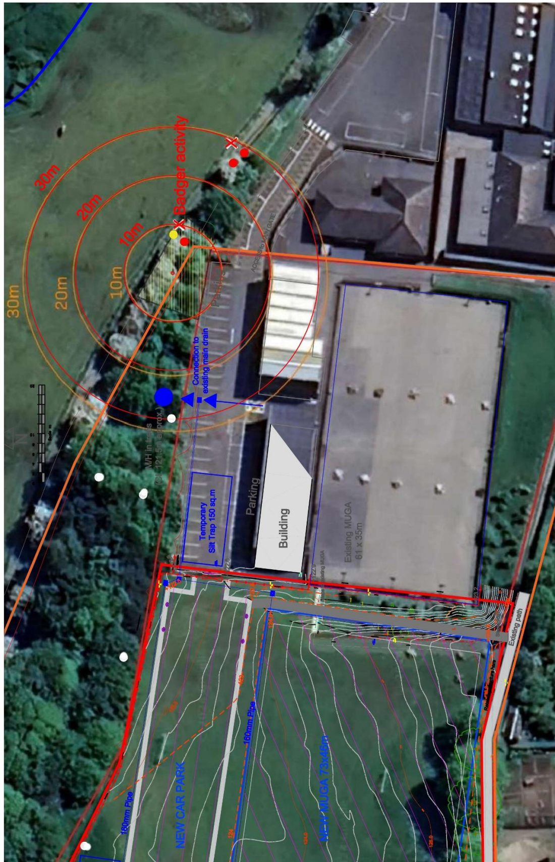
Fig. 2 – The located badger sett, possibly disused, and distances by radius to the edge of the working area, new drain connection to existing in the current car-park.
