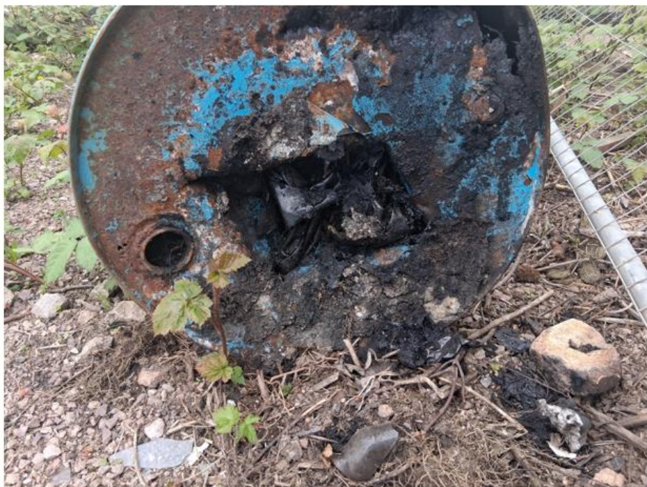
Photo No.9: Leaking oil barrel with strong olfactory evidence of hydrocarbons noted in northern yard area
