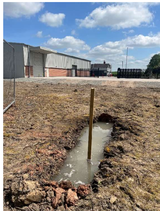
Figure 5: Test hole filled to 100%
