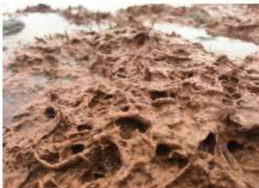
Close up FlocMat showing accretion of silt
