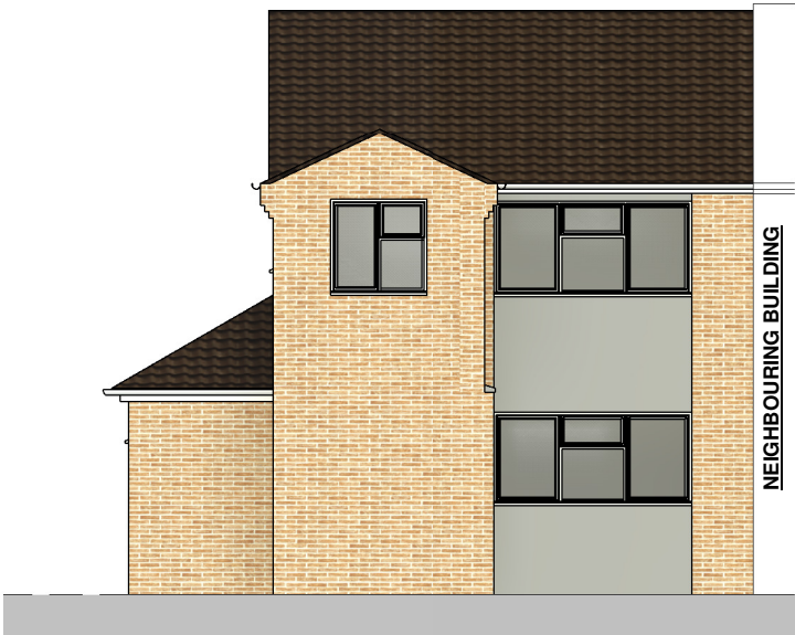
Proposed Front Elevation Scale @ 1:100
